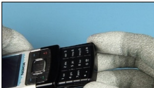
10. Gently press both edges together until a gap appears at the end of the KEYMAT.
